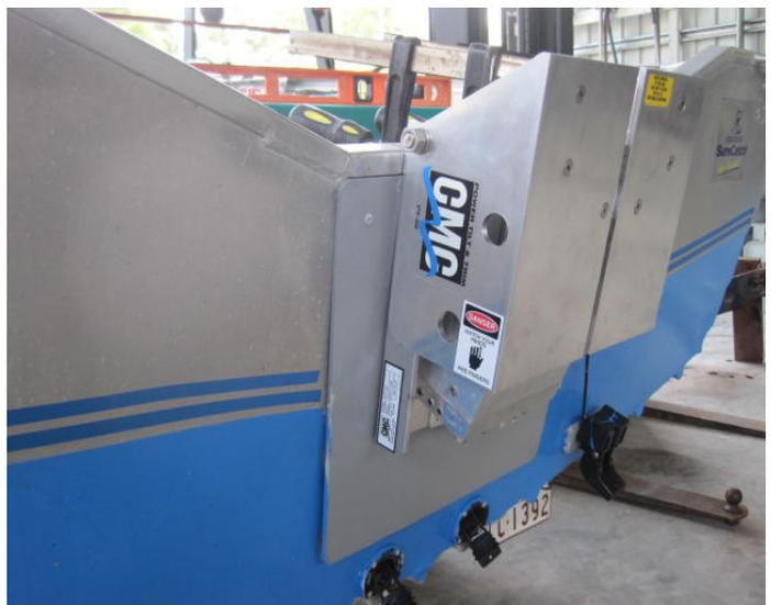
Whilst the clamps hold the unit in place, mark the hole positions with a cut off pencil
