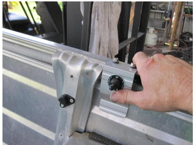
Now your PT-35 is all mounted up and ready to have the outboard fitted. At this stage you would have finished mounting the switch, positioned the relays and extra wiring in the battery box, or where-ever you decide to place it.
