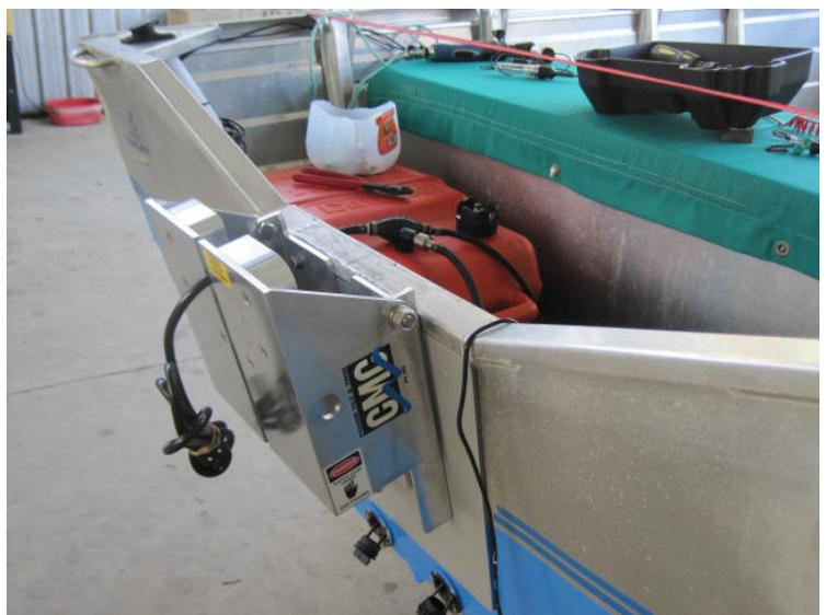
At this stage I like to drill a 3-4 mm hole in the plate so that a zip tie can be used to hold the electrical lead in position.
