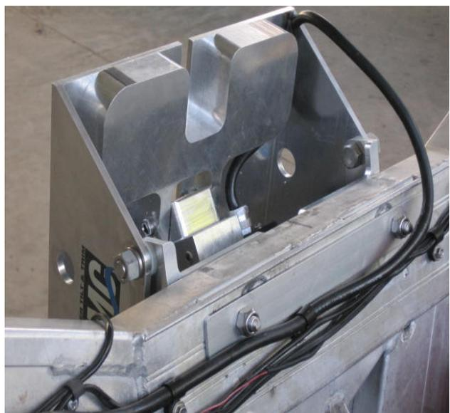
Mount the outboard, position it evenly on the plate and do the clamps up.
