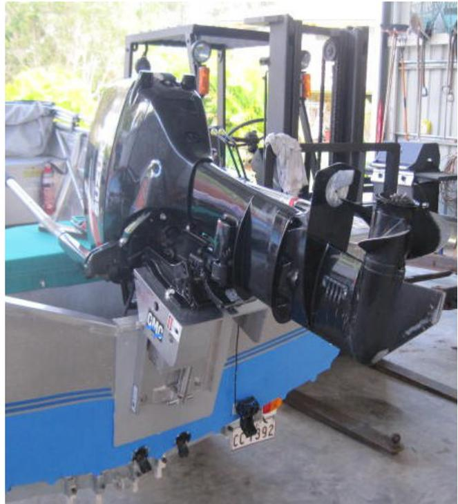
Now tilt the outboard back down again so that you can easily drill through the trim and tilt plate, using the outboard as a template. These will be the holes for the bottom bolts on your outboard, locking it into place.
