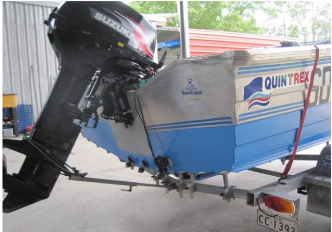
Start by removing the engine from the transom, in this case a 1 inch block was spacing the outboard up, remove this at the same time. Use 2 "G" clamps to position the PT-35 using the transom as a guide. Mark off where you want the unit to be fitted. Mark the centre of the transom as a guide, small adjustments can be made later.
