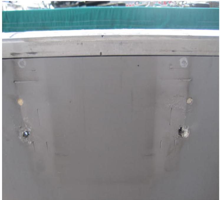
Once you have your bolt holes drilled, fit the bolts, place the unit into its correct position, tighten the bolts using nylocks or stainless spring washers. I used a strap washer with nylocks for the top fasteners in this case, it lends support and makes a neat job.
