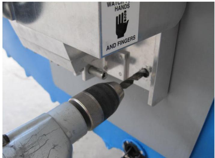
Followed by this one, although you may only be able to mark the hole position with the drill as the chuck may strike the actuator if you have a short drill.
