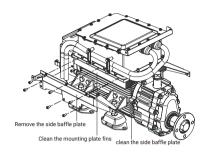
Clean the side baffle plate, motor and driver mounting plate
