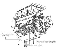
3. Clean the bottom baffle plate and motor
