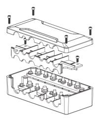
Figure 4-1 The disassembled bus bar
