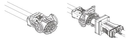
Figure 4-9 High voltage interlocking plug
