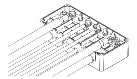
Figure 4-3 Negative wiring position of the bus bar
