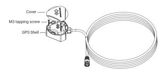
Figure 4.21 GPS External Module Mounting Method 2
