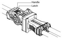
Figure 4.15 High-voltage interlock pconnector - Installation step 5
