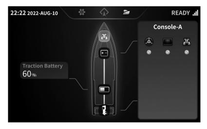
When the accessories fail, the icon will turn orange or red. Click the fault icon to view the detailed fault.
