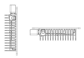
Torque shall be 6 N.m when using self tapping bolts fixed the DCDC on the hull.
