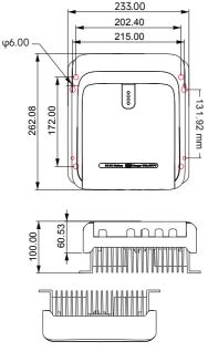
Product dimensions: 233\*262\*100mm Mounting dimension: 215\*132mm Fixing hole position:  $\phi$ 6mm
